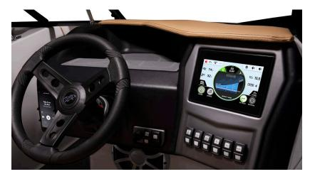
**FUEL GAUGE:** Indicates the approximate amount of fuel in the tank. The ignition switch must be in the RUN position to activate the gauge.
